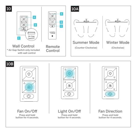
**Fan On/Off**: Press and hold  $\mathfrak{B}$  button for 4 seconds. The LED on the remote will flash green and all connected fans will beep to indicate the message has been received. All fans will turn off. This will bring all fans controlled by the remote into sync.
