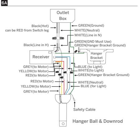
Follow the steps above to connect the fan to your household wiring. Use the plastic wire nuts with your fan. Secure the plastic wire nuts with electrical tape. Make sure there are no loose strands or connections.
